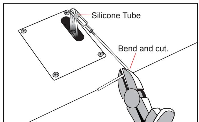
Insert the 90 degree bend down through the hole in the control horn. Install one nylon snap keeper over the wire to secure it to the control horn. Install the control horn retaining screw and remove the masking tape from the aileron.
