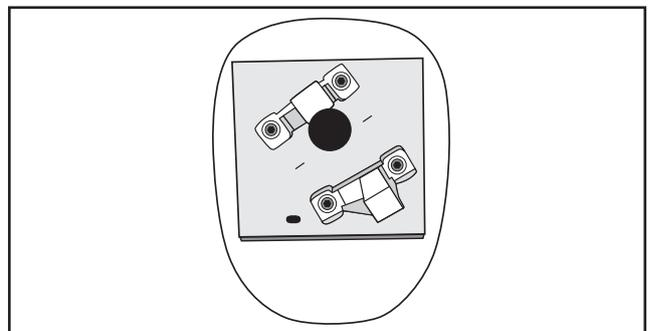
Locate the long piece of wire used for the throttle pushrod. One end of the wire has been pre-bend in to a "Z" bend at the factory. This "Z" bend should be inserted into the throttle arm of the engine when the engine is fitted onto the engine mount. Fit the engine to the engine mount using the screws provided.
