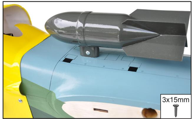
**INSTALLING PLASTIC BOMB FUSELAGE**
