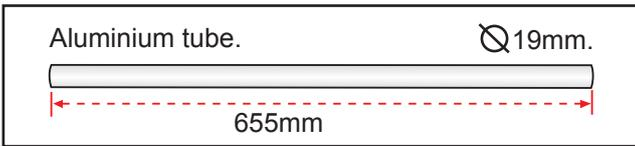
\*\*\* Test fit the aluminium tube dihedral brace into each wing haft. The brace should slide in easily. If not, use 220 grit sand around the edges and ends of the brace until it fits properly.
