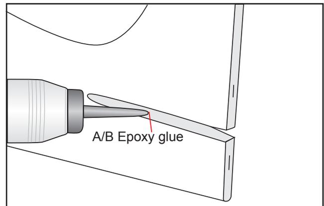
After the epoxy has fully cured, remove the masking tape or T-pins used to hold the stabilizer in place and carefully inspect the glue joints. Use more epoxy to fill in any gaps that may exist that were not filled previously and clean up the excess using a paper towel and rubbing alcohol.
