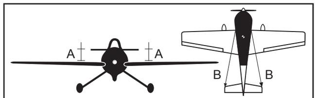
□ 4) Check the fit of the horizontal stabilizer in its slot. Make sure the horizontal stabilizer is square and centered to the fuselage by taking measurements, but don't glue anything yet.
