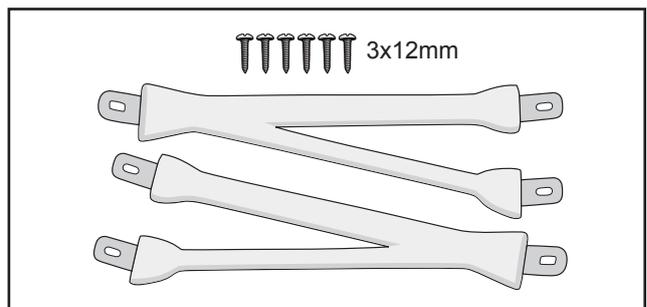
□ 2) Mark the locations of the two mounting screws. Remove the tail wheel bracket and drill 2mm pilot holes at the locations marked.
