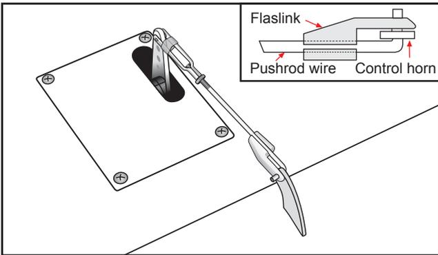
Repeat the procedure to install the second aileron linkages in the opposite wing half.
