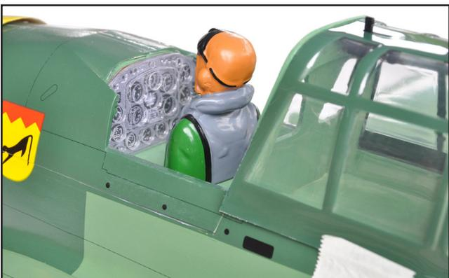
Position the canopy so the rear frame on the canopy is aligned with the rear edge of the cockpit opening. Use canopy glue to secure the canopy to the canopy hatch. Use low-tack tape to hold the canopy in position until the glue fully cures. Wrap the tape completely around the canopy hatch.
