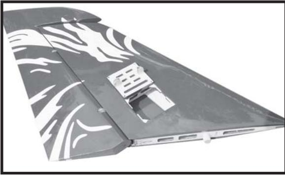
Rudder servo install as same as method of elevator servo.
