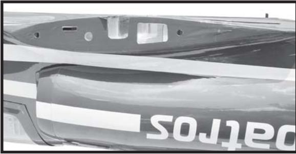
□ 2. Attach the carbon tube into the fuselage.
