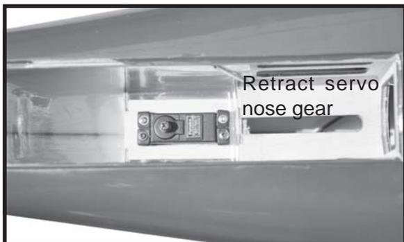
**INSTALLING RETRACT NOSE GEAR.**
