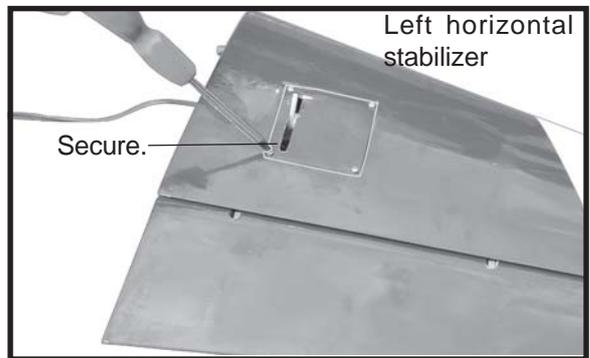
**ELEVATOR CONTROL HORN INSTALLATION.**
