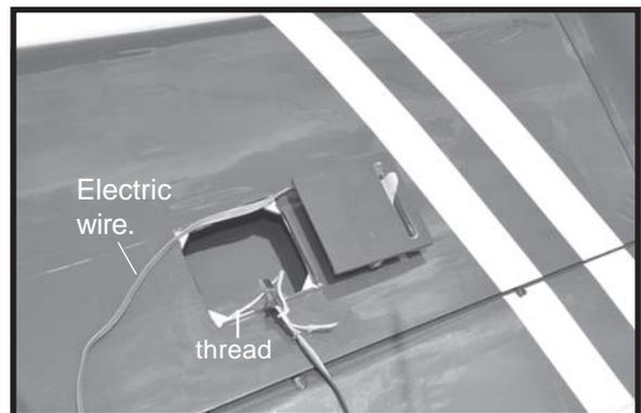
□ 5. Instal servo tray with aileron servo into the wing as same as picture below.
