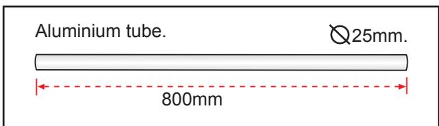
\*\*\* Test fit the aluminium tube dihedral brace into each wing haft. The brace should slide in easily. If not, use 220 grit sand around the edges and ends of the brace until it fits properly.
