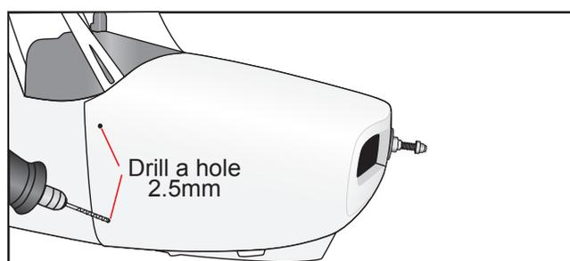
Drill four 2.5mm pilot holes through both the cowl and the side edges of the firewall. Using a 3mm drill bit, enlarge the four holes in the cowling.
