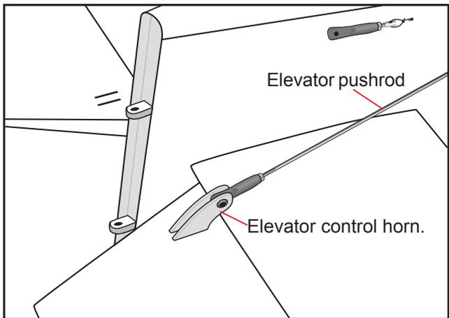
Repeat the procedure to install the control horn on the opposite elevator.
