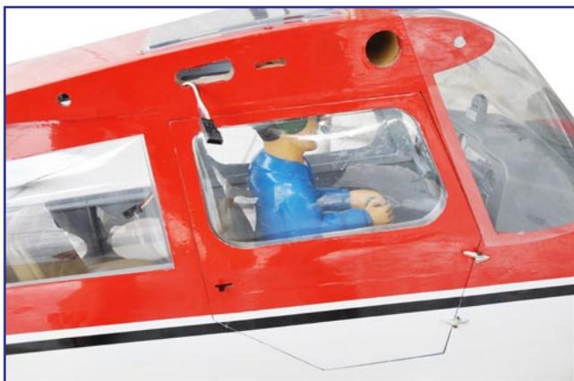
Attach the aluminium tube into the fuselage.
