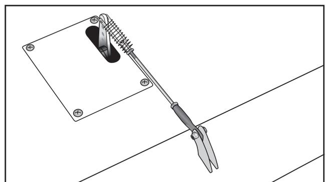
After both linkages are completed. connect both of the aileron servo loads using a Y-harness you have purchased.
