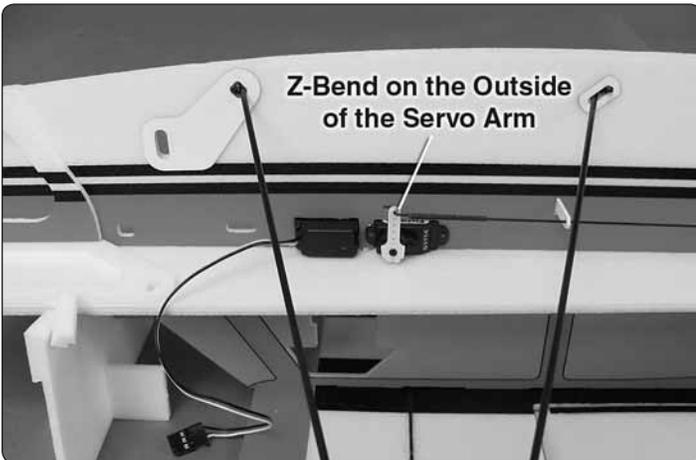
❑ 9. Remove the servo arm from the rudder servo and insert the z-bend in the outer hole of the servo arm. The pushrod should be to the outside of the servo arm, away from the fuselage. Re-install the servo arm screw in the servo.
