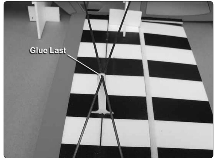
❑ 9. Once the glue has cured, glue the carbon rods to the brace supports.
