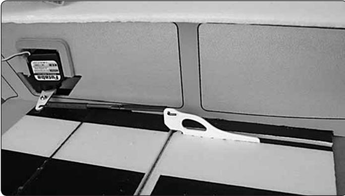
❑ 7. Insert an **ABS aileron control horn** onto the end of both aileron pushrods. Insert the aileron control horns in the slot in both ailerons. With the transmitter switched on and the aileron servo arm centered, check that both ailerons are centered. If they are not, adjust the length of the aileron pushrods as needed. Then, glue the aileron control horns in the aileron. Again, check that the ailerons are centered and apply a drop of thin CA to the end of the heat shrink tubing.
