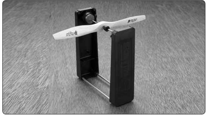
Carefully balance your propeller and spare propellers before you fly. An unbalanced prop can be the single most significant cause of vibration that can damage your model. Vibration of props on small models can cause a loss of power, but vibration may also damage your radio receiver, battery and possibly the motor bearings.
