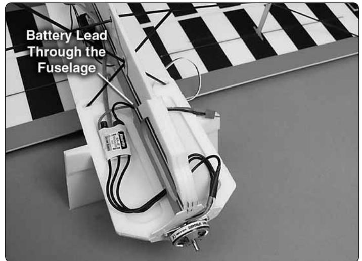
❑ 4. Place a piece of hook (rough) material under the fuselage, close to the front. Route the motor leads through the fuselage and connect them to the motor. Attach the ESC to the hook material.
