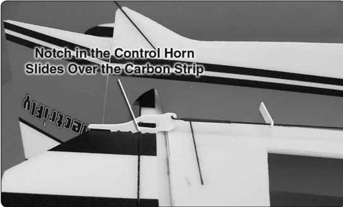
❑ 8. Insert the z-bend in the **elevator control horn**. Insert the control horn in the slot in the elevator. The notch in the control horn should slide over the carbon fiber strip in the elevator. If the control horn will not fit over the carbon fiber strip, use a sharp hobby knife to remove the excess glue from the slot. **DO NOT** glue the horn to the elevator until told to do so.
