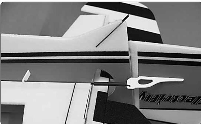
❑ 10. Slide the **black heat shrink tubing** over the aft end of the rudder pushrod. Insert the z-bend wire into the hole in the **rudder control horn** from the bottom. Slide the other end
