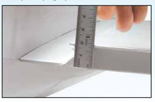
Elevator: 27mm each way at tip of elevator, with 20% exponential
