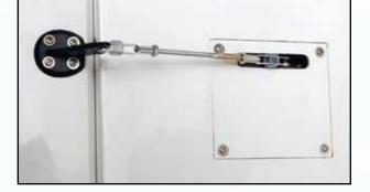
Fit the rudders to the tail booms, installing the hinges in a similar manner to that illustrated for the elevator, note that the rudders are handed and have hard points for the control horns on the inboard sides, and the rudder servos are consequently fitted on the inboard sides of the booms
