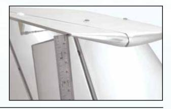
Rudder: 60mm each way at base of rudder, with no exponential
