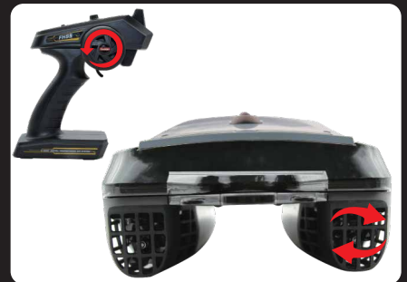
C: Rotate transmitter wheel in anticlockwise direction, left propeller stop, right propeller rotate as photo shown. This control drive boat steering to left
