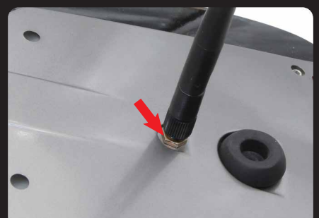
I: Install the antenna on mounted antenna stand. Now complete the installation of fish finder.
