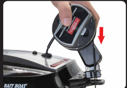
E: Mount the cable wheel at rear support of boat as photo shown.
