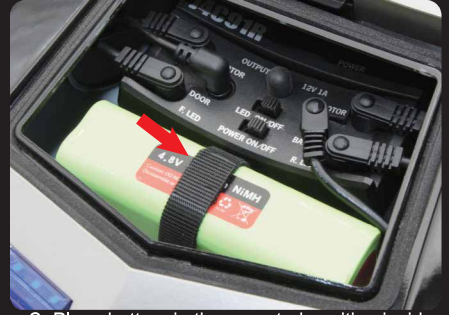
C: Place battery in the mounted position inside cabin. Secure battery with velcro strap.
