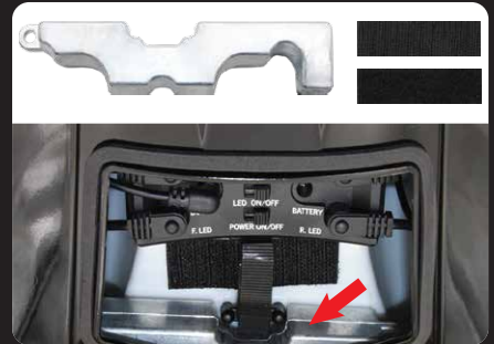
B: Use stickers on balance weight to mount balance weight inside the forward of carbin.
