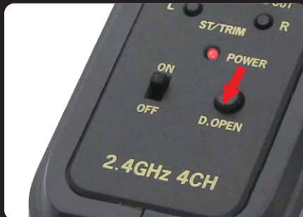
G: Push transmitter button "D.OPEN", the blinking red light will change to staying bright.
