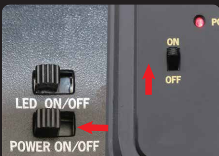
A: Firstly switch on transmitter, then open hatch on cabin, switch on receiver box power, make sure transmitter red light and receiver box blue light are staying bright.
