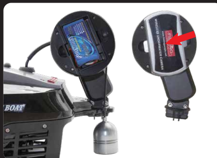
G: Install battery inside cable wheel and close battery compartment.
