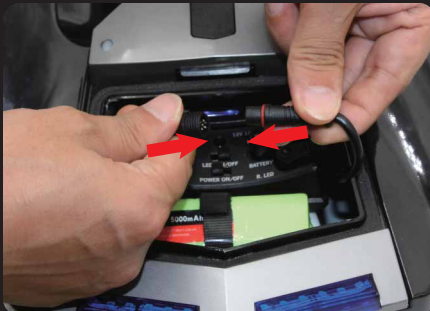
C: Use camera cable to thread through the big hole on boat handle, then reach to the forward cabin. Connect with receiver box's waterproof connector.
