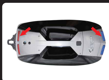
B: Forward Blue LED light, Rear Red LED light. To tell direction when drive boat.
