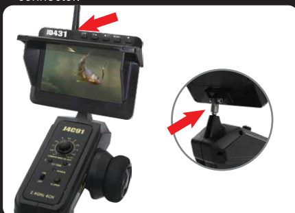
F: Mount display on transmitter as photo shown, Switch on display.
