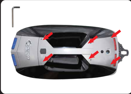
A: Used supplied Allen Key to loose the 6pcs screw on boat handle.
