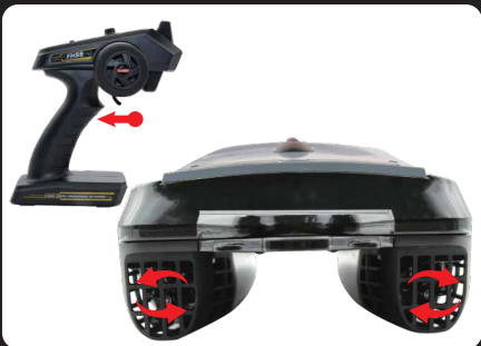
A: Pull trigger backward, left and right propeller rotate as photo shown. This control drive boat forward. propeller rotate speed will change proportionally base on how you pull trigger.
