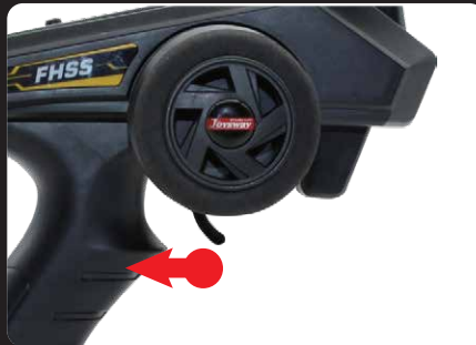
E: Pull trigger back to rear end, then allow trigger back to neutral position slowly.
