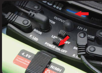
H: Switch on "POWER" on receiver box. Now receiver box blue light will be staying bright. This means BIND process complete successfully.
