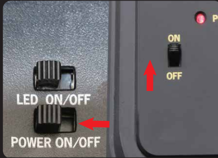
E: Switch on transmitter firstly (Transmitter red light on), then switch on "POWER" on receiver box (receiver box blue light stay bright) F: Now transmitter connect with boat, proceed next step testing.
