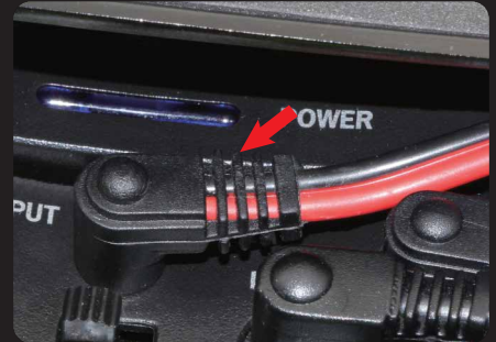
C: Use supplied specialized connector to connect with power cable of transducer. Connect the transducer's modified connector with power socket(12V 1A) from receiver box.
