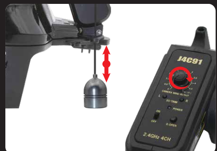
I: Use the transmitter's camera rotate knob to control the camera cable length. (NOTE: Cable line total length 5.5meters, control cable length 5meters)
