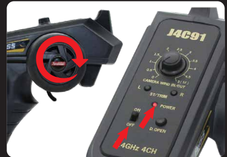
C: Rotate the transmitter wheel to right end and hold, Switch ON transmitter, red light is on. Rotate wheel back to neutral position slowly, red light is blinking.
