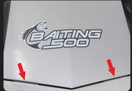
G: Follow photo to install back the hatch on cabin. Press down hatch align to cabin two mounted slot.
