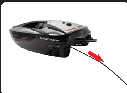
B: Place boat evenly, pull line straight out from hopper.
