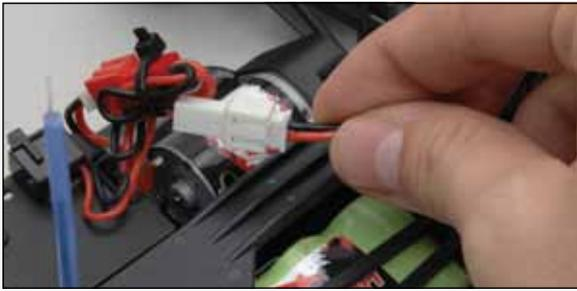
Plug the battery connector on the ESC into the battery connector on the battery. As a safety feature, the connectors can only be plugged in one way.
