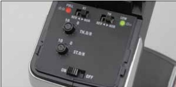
Lift up the protective cover from the transmitter and turn on the transmitter by moving the switch left to its on position. Both the red and green transmitter LEDs should light up.
