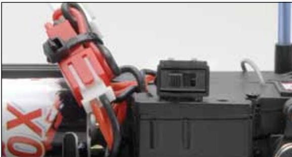
**IMPORTANT** Lift the car off the ground before turning on the receiver to ensure that if the motor turns on when you turn on the receiver, the car won't drive away.
