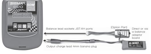
The main battery leads must be connected along with the balance lead connector as shown, before charging your battery.
