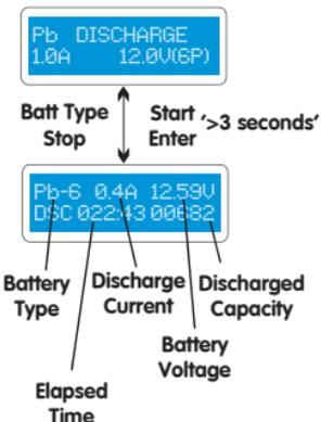
Set the discharge current on the left and final voltage on the right. The discharge current ranges from 0.1 to 1.0A. To start the process, press and hold the START/ENTER key for more than 3 seconds.
