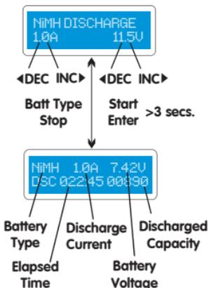
Set the discharge current on the left and final voltage on the right. The discharge current ranges from 0.1 to 1.0A and the final voltage ranges from 0.1 to 25.0V. To start the process, press and hold the START/ENTER key for more than 3 seconds
