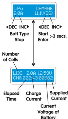
You can set up the charging current and the voltage of the battery pack being charged. As you press the START/ENTER button, the voltage confirmation will be displayed. Then, if you confirm the voltage and current, press START/ENTER button again to start charging.
