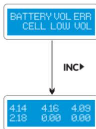
The processor found that the voltage of one cell in the Lithium battery pack is too low.
