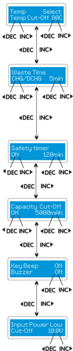
The 3-pin port on left side of the unit is used for the temperature sensor. The temperature probe must be attached to the surface of the battery in order for this to function. You can set the maximum temperature at which the charger should allow a battery to reach during the charge process. Once a battery reaches this temperature during charge, the process will be terminated to protect the battery.
