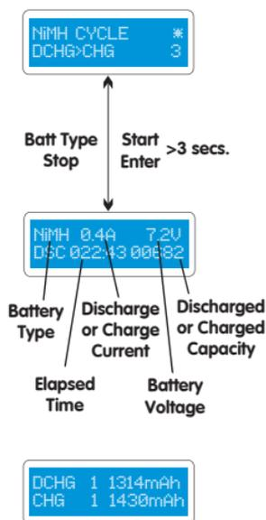
Set the sequence on the left and the number of cycles on the right. You can use this function for balancing, refreshing and breaking-in the battery. To avoid raising the temperature of the battery, there will be a brief cool-off period (already fixed at 'User setting') after each charge and discharge process. The cycling number ranges from 1 to 5.
