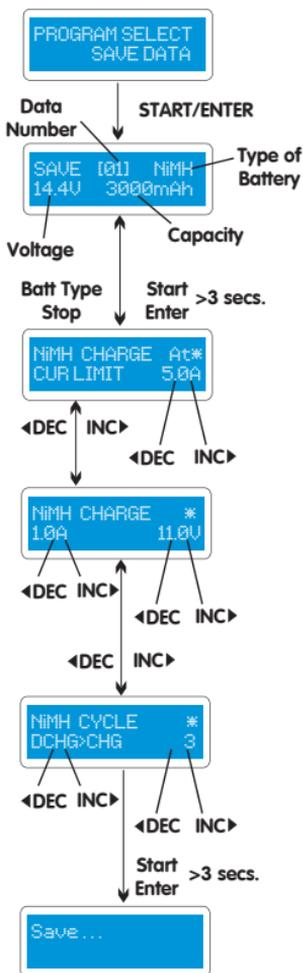
The parameter values set up in this screen do not affect the charge or discharge process, they only represent the specification of the battery. The following screens will automatically display values/settings matched with the battery type you set up. The example shows a NiMH battery pack of 12 cells and 3000mAh capacity.
