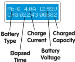
The screen displays the state of charging process. To stop charging at any time, press the BATT TYPE/STOP key once. The audible sound indicates that you ended the process.
