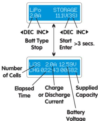
You can set up the current and the voltage of the battery pack to be charged. The current will be used for charging or discharging the battery to reach the required 'storage' voltage level.
