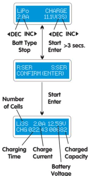
The left side of the first line shows the type of battery you selected during the users setting. The value on the left side of second line sets a charge current and the value on the right side of second line sets the voltage of the battery pack. After setting the current and voltage press START/ENTER key and hold for 3 seconds to start the process. (Charge current: 0.1~6.0A, Voltage: 1-6 series for instance)
