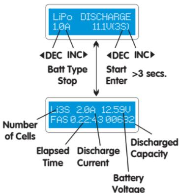
The value of the discharge current on the left side of screen should not exceed 1C for maximum safety. The final voltage on the right should not be under the voltage level that is recommended by the battery manufacturer for deep discharging.
