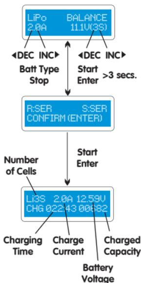
The value on the left side of second line sets the charge current and the value on the right side of second line sets the total voltage of the battery pack.
