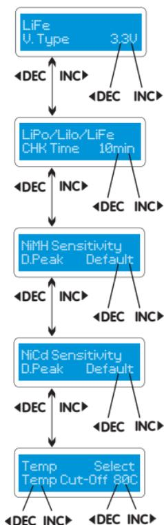
This screen displays the nominal voltage of a Lithium battery. There are three kinds of Lithium battery; LiFe (3.3V), Lilon (3.6V) or LiPo (3.7V). This is very important, so make sure you check the battery carefully and select the correct program regime. If you select an incorrect value/regime, the battery can explode during the charge process!
