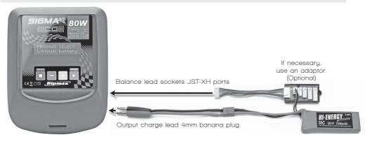
The main battery leads must be connected along with the balance lead connector as shown before charging your battery. If using crocodile clips make sure they are unable to touch together!
