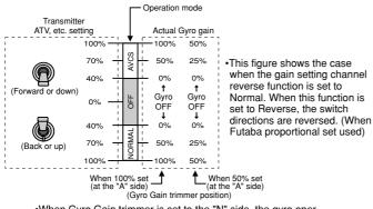
•When Gyro Gain trimmer is set to the "N" side, the gyro operates in the normal mode at both side of the switch directions.
