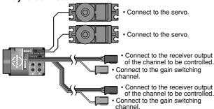
When there is no vacant channel that can be used for gain switching, Standard setting" cannot be performed. See "Beginner setting" When there is one vacant channel only, use a branch cord to simultaneously switch the gain of two axis
