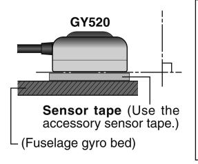
**[IMPORTANT]** Install the sensor so that the bottom of the gyro is perpendicular to the main shaft axial direction. Offset of this axis will also react in the roll and pitch directions.
