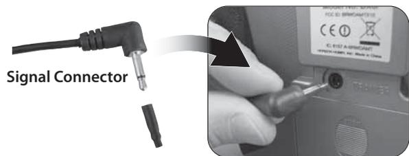
B. Remove the protective boot from the signal connector. Carefully insert the signal connector into the transmitter's trainer / D.S.C. jack. The Tx logic circuit will turn on automatically at this time.
