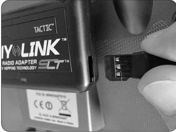
C. Insert the power connector into AnyLink's INPUT jack. Confirm that AnyLink's LED turns on at this time.
