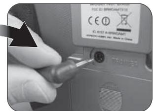
B. Remove the protective boot from the signal connector. Carefully insert the signal connector into the transmitter's trainer / D.S.C. jack. The Tx logic circuit will turn on automatically at this time.
