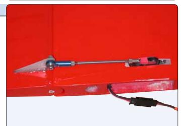
Section: Aileron/Flap Linkage
