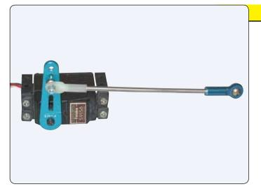
Prepare your flap servos by fitting their rubber grommets and ferrules, then screw them to the moulded right-angled mounting brackets as shown. Note that M3 screws are used to screw the servos to these brackets. Some servo ferrules may be too small to accept these screws, so will have to be changed to a suitable type. Due to the size of the flaps, we recommend using heavy duty aluminium servo horns. Make up the flap linkage as shown and screw to the servo horn.
