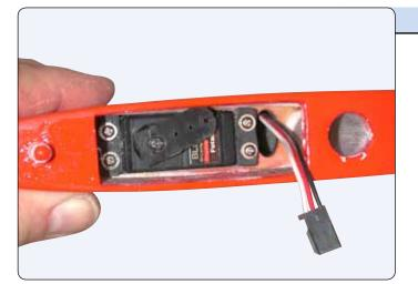
Assembly begins with the fitting of your choice of elevator servo in its pre-fitted mount in the first tailplane half. Note the orientation of the servo. Use the mounting screws, grommets and brass ferrules supplied with your servo and ensure that the lead is drawn out of the tailplane through the opening in the mount. Temporarily fit a servo control horn as shown.
