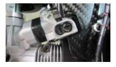
•Low needle :For adjustment from idle to hovering (it will slightly affect the general flying also)
