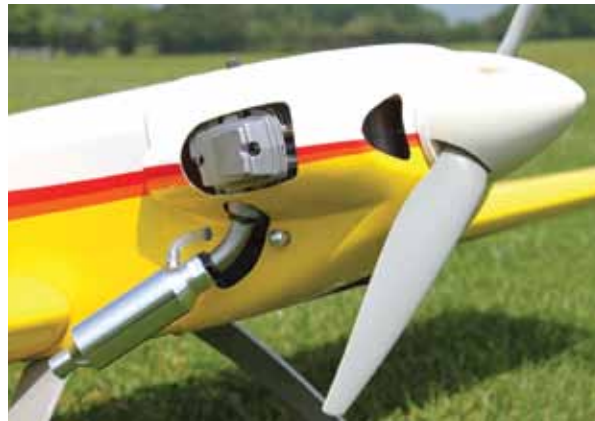
The simple, strong, fuss-free dural u/c is easy to fit and absorbs the shocks nicely.
